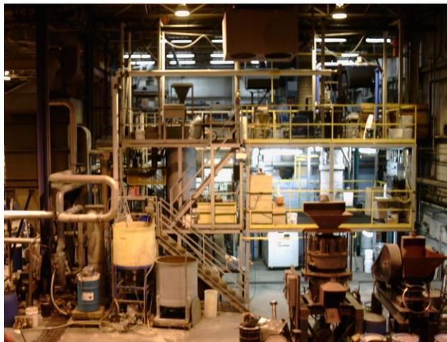
On site equipment includes various crushers, mills, screens and drying ovens for feed preparation. Laboratory facilities are available to allow simple analytical tests to be undertaken such as screen size analysis, moisture content, loss on ignition (LOI) and particle density and bulk density. Other analyses are contracted out to Bodycote ORTECH that is located in adjoining facilities or samples can be returned to clients for their own in-house analysis.
