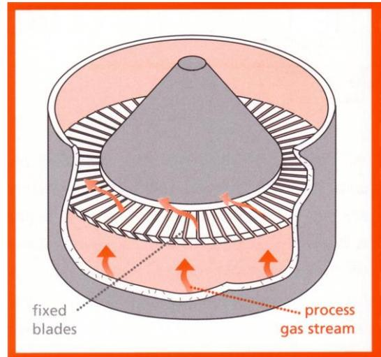
*Process gas flow through fixed blades gives toroidal particle motion. By producing an annular processing region with toroidal mixing, material is continuously passed through the base of the bed where the high heat and mass transfer occurs. This ensures uniformity of processing*
