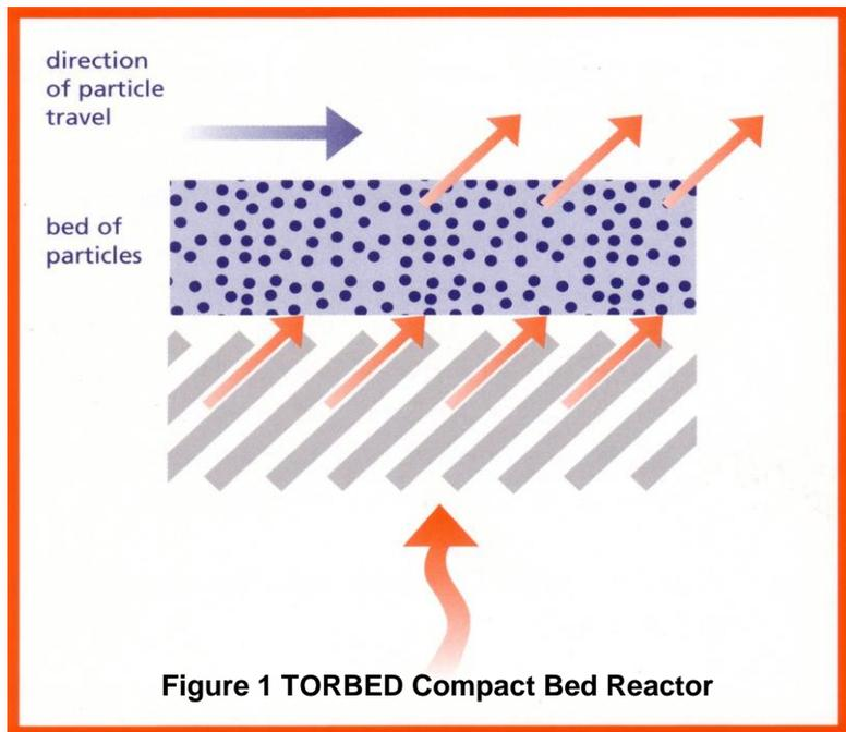
Figure 1 TORBED Compact Bed Reactor
