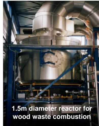
1.5m diameter reactor for wood waste combustion
