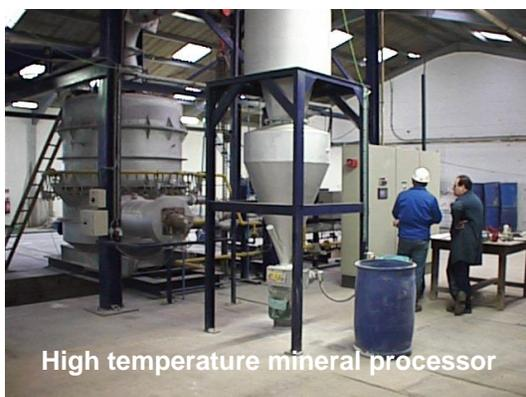
The TORBED reactor has shown itself to have unique capabilities in this application in producing higher quality, lighter and more consistent product with lower energy consumption. High heat and mass transfer and precision of control with the TORBED reactors have provided these advantages. Most important, the TORBED process provides more saleable product per unit of raw material fed i.e., a higher yield.
