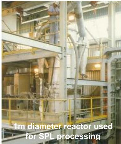
1m diameter reactor used for SPL processing
