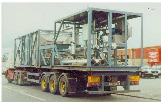
In 1993, a pilot plant capable of processing 150 kg/h of oil-contaminated solids was fully tested at BP's Sunbury laboratories. A consortium of oil and gas exploration companies then funded the further development of the TORBED reactor as a **transportable de-oiling plant** for eventual off shore use. This plant demonstrated the capability of stripping hydrocarbons from solids in a controllable manner.
